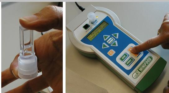
Agitate the test tube, inverting it.
