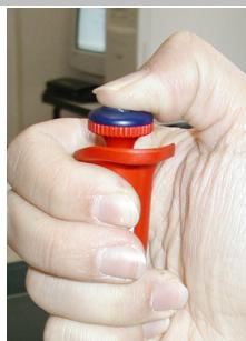
Immerse the tip into the liquid in the test tube and pump the piston up and down 2-3 times by using the thumb.
