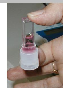
Close the test tube with its cap and agitate, inverting it.
