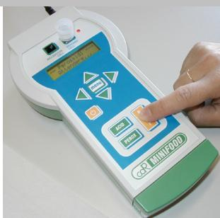
Insert the test tube in the reading cell and press **ENTER**.
