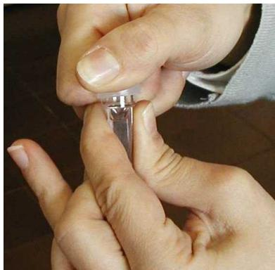
The caps has be opened carefully by putting pressure to the right and then to the left. Do not touch the internal parts (soaked) of the cap with the hands.
