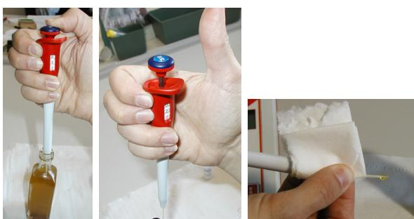
Take 2.5  $\mu$ l of the sample: immerse the tip of the tip of the pipette into the oil with the piston lowered. SLOWLY lift the piston keeping the top of the tip immersed in the sample.
