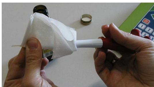
It is fundamental for making correct analysis that the tip is clean outside: clean it with adsorbent paper as shown.
