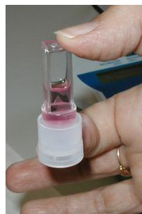
Close the test tube with its cap and agitate, inverting it.
