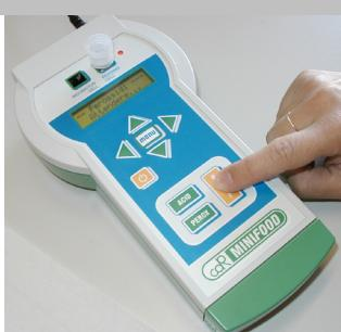
Insert the test tube in the reading cell and press **ENTER**.
