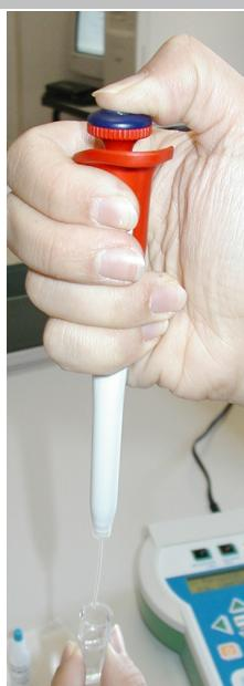
Immerse the tip into the liquid in the test tube and pump the piston up and down 2-3 times by using the thumb.
