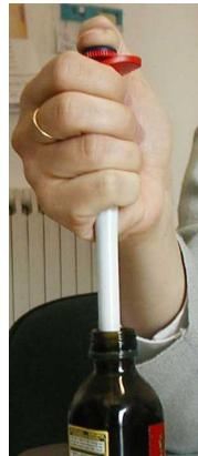
When taking the sample always agitate it, inverting the container with the sample and immerse the tip keeping the piston lowered.
