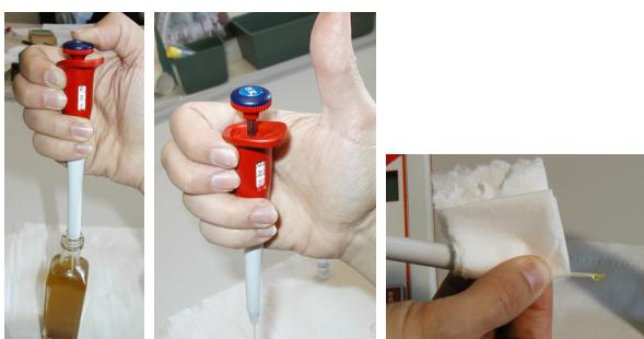
Take 2.5  $\mu$ l of sample for Low Acidity or 1.25  $\mu$ l for High Acidity: immerse the tip of the pipette into the oil with the piston lowered. SLOWLY lift the piston keeping the top of the tip immersed in the sample.
