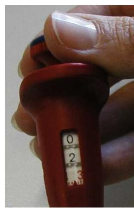
Before making an analysis, check that the volume in the pipette is correct.
