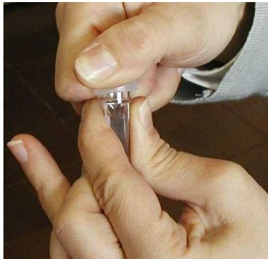
The caps must be opened carefully by putting pressure on the right and then left. Do not touch the internal parts (soaked) of the cap with the hands.
