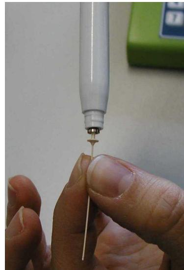
Do not leave a space between the tip and the pipette: push it fully in.
