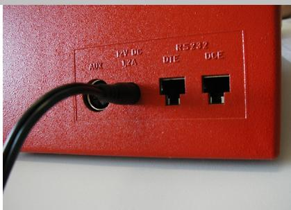
To switch on the instrument insert the plug...
