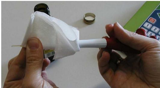
The cleanliness of the tip is fundamental for making a correct analysis: clean it by sliding the tip on paper.
