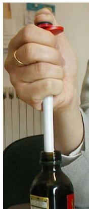
When taking the sample, always agitate by inverting the container with the sample and immerse the tip keeping the piston lowered.
