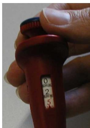
Turn the piston until the required volume is centred by the arrow (e.g. 5 $\mu$ l = 050).
