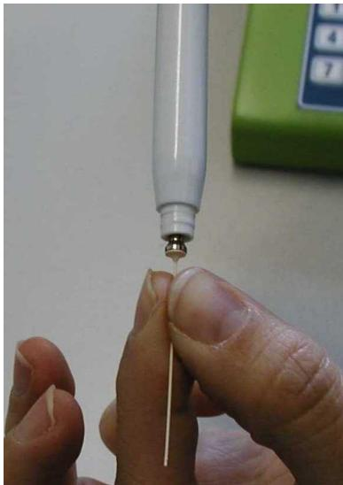
Insertion of a new tip: push the piston with force right to the end of its travel so that the tip adheres well.
