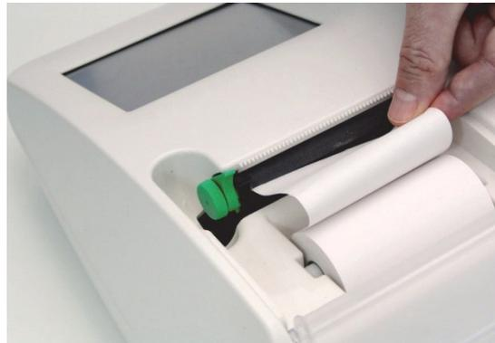
Pull up the green lever on the printer to release the black roller and insert the paper under the printer roller.
