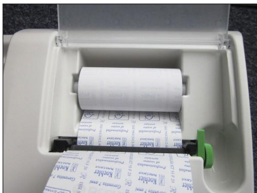
Figure 42 Printer - change of thermal paper
